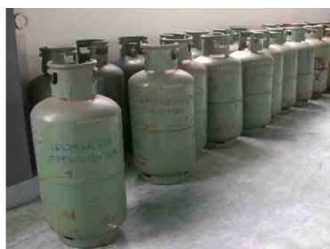
Refillable cylinders each holding 25 kg of HCFC-22
