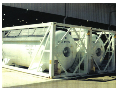
Refillable ISO tanks each holding about 30 tonnes of HCFC-22
