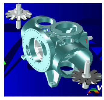
Recent Compressor development offers high pressure compressors with balanced radial and axial forces suitable for condensing ammonia at 95°C
