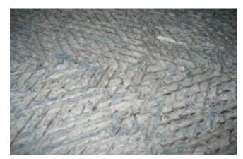
Limescale can block your heat exchanger.
