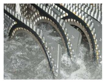
A combination of heating and turbulence (enabled by airbubbles) results in more efficient cleaning.
