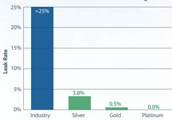
Average amount of refrigerant leaked in stores of each certification level versus industry average, up to December 2011. Based on stores with at least 12 months of leak data.
