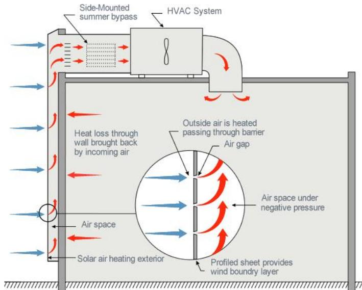
**Schematic of a typical solar air heating system**
