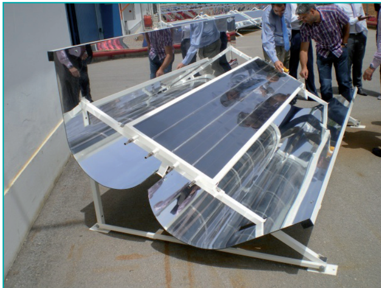
Figure 28 - Non tracking TVP high vacuum flat-plate collector with mirrors which can reach temperatures up to 400 °C. Source: AEE INTEC
