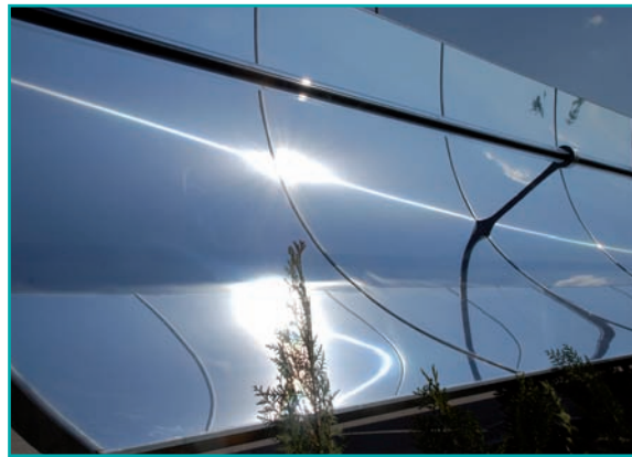
Figure 27 - Concentrating parabolic troughs collector. Source: Solitem
