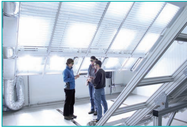
Figure 36 - Dynamic solar simulator of the Research and Testing Centre for Solar Thermal Systems (TZS) at ITW, University of Stuttgart, Germany Source: ITW
