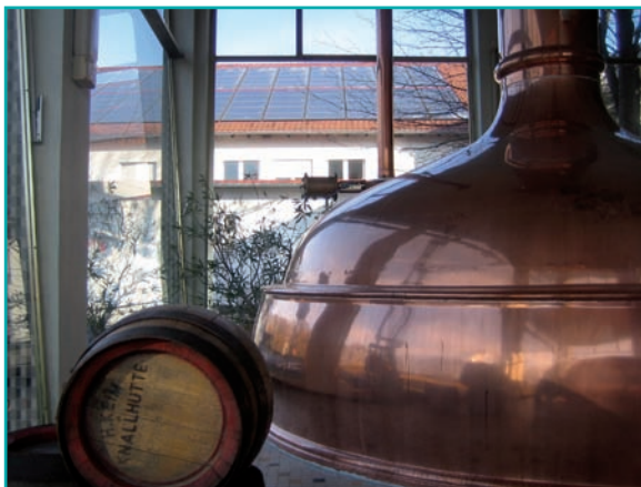
Figure 13 - Mash tun of the Hütt Brewery in Kassel (Germany). In the background, solar heating system (155m 2 flat plate collectors) integrated into the hot water buffer of the brewer (pilot plant realized within project “SOPREN – Solar process heat and energy efficiency”) Source: Institute of Thermal Engineering, University of Kassel
