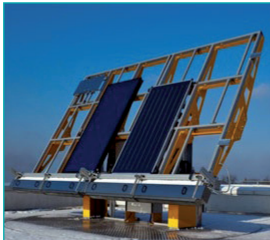
Figure 37 - Precision tracker to characterize façade, large-area and concentrating collectors. Source: Fraunhofer ISE
